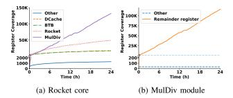
Fig. 2: DIFUZZRTL's register coverage breakup for Rocket.
