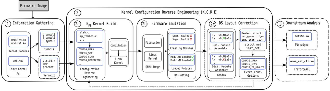
Figure 1: System overview of *FirmSolo*: The dashed boxes indicate that a step or information are optional. Also while stage 3 is not part of *FirmSolo*, we feature two representative downstream analysis.
