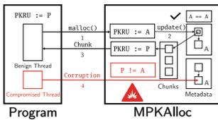
**Fig. 2.** Architectural overview of MPKAlloc.
